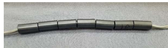
FIGURE 86 Feed the cut end of the CAT3 cable through 7 in-line Ferrite Beads.
