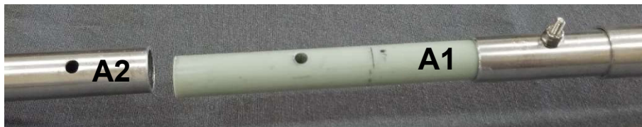
FIGURE 24 Align A2 tube end relative to A1 as shown.
