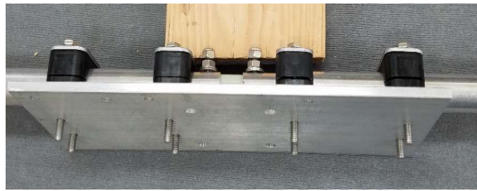
FIGURE 17 Rotate plate edge on surface until input terminals rest on support wood block with inserted HEX bolts protruding.
