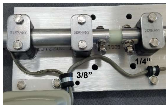
FIGURE 95 Mounting junction box plate and P-clamps to element plate and input cable management.
