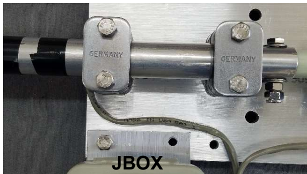
FIGURE 94 Align 2 holes of the junction box mounting plate with element plate holes and insert one (1) 1/4"-20 bolt and hardware at the corner.
