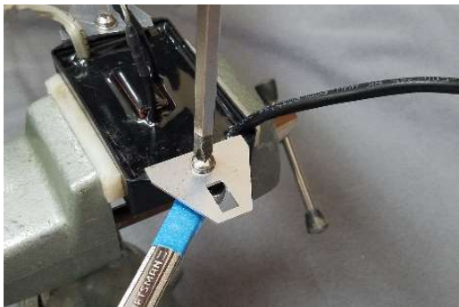
FIGURE 58 Phillips screw driver holds the #8 screw, as the #8 lock nut is tightened with open end 11/32" wrench.
