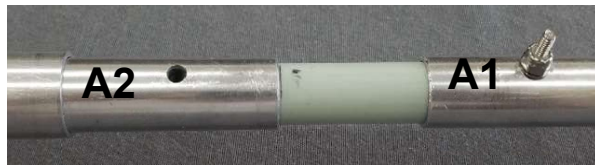
FIGURE 27 A1 and A2 after hole alignment
