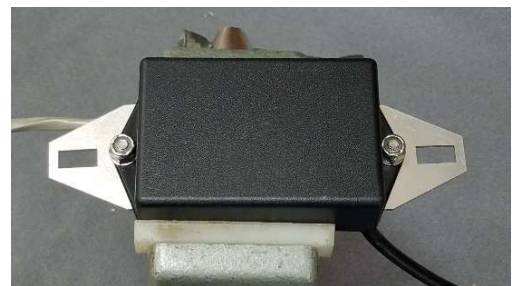
FIGURE 59 Finished attached module support plates to module.
