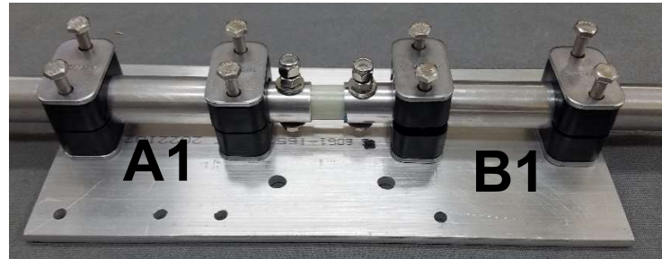
FIGURE 15 Repeat process of FIG. 14 for remaining 3 clamp assemblies. Press down on all HEX bolts to insure fully inserted through element plate.
