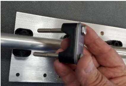
FIGURE 14 Insert HEX Bolts through top portion of clamp/plate and then through bottom portion of clamp/plate and element plate.
