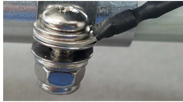
FIGURE 79 Loose connection view of FIG. 78 [ring connector to P-clamp contact].
