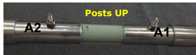
FIGURE 30 Finished coupling of sections A1 and A2 after tightening of hardware.
