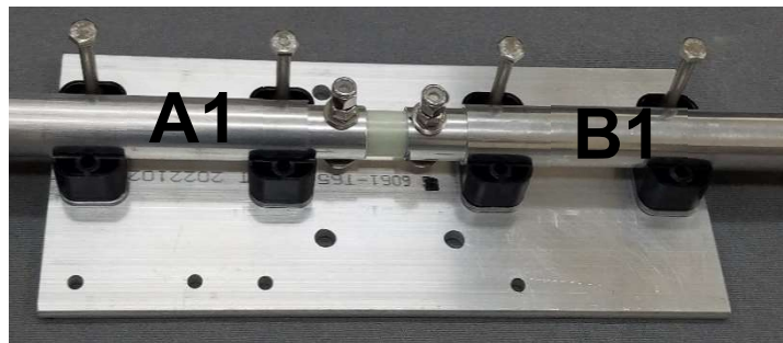
FIGURE 11 Use of A1/B1 sections to align half clamps.
