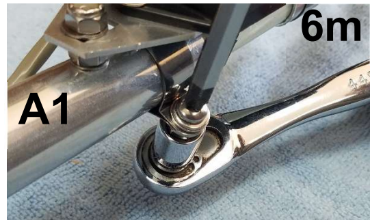
FIGURE 81 A socket wrench and a screw driver is used to tighten hardware connection.
