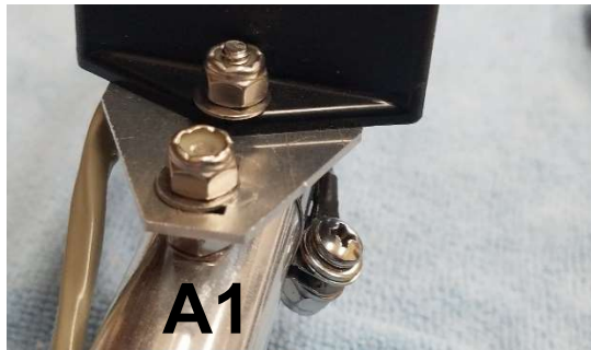
FIGURE 80 Ring connector attached to P-clamp at an angle for screw driver access.
