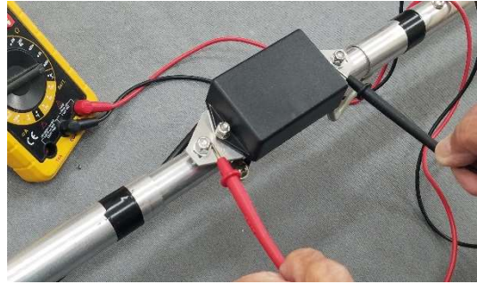
FIGURE 119 Module resistance measurement across the support plates (or across the element sections).
