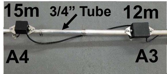
FIGURE 74 15m module after routing the cable from both modules shown UNDER the element.
