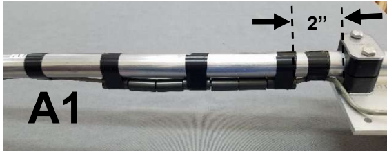
FIGURE 87 Seven Ferrite Beads tape wrapped to A1 section and CAT3 cable routing.
