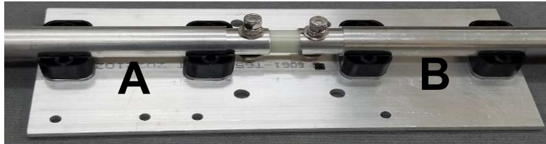
FIGURE 13 All HEX bolts removed after pre-alignment procedure of FIGs 11 and 12 .
