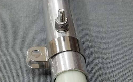
FIGURE 63 Proper placement of P-clamp with sharp bend contact leg UP.
