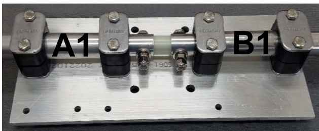
FIGURE 20 Rotate element input terminals as shown.
