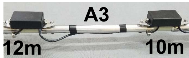
FIGURE 90 Final taped cable under section A3 from 12m to 10m module.
