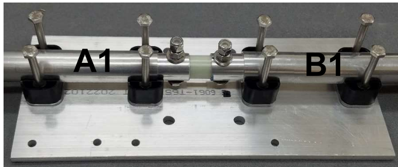
FIGURE 12 All HEX bolts are pushed through to bottom surface to ensure ALL clamp/standoff plates are aligned through bottom element plate.
